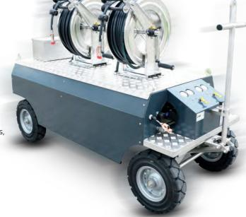
14594. The ARGO is fitted with an integral stainless steel control panel as standard, that comes with two 0-10 bar reducer valves and a high- and low-pressure manometer, as well as a mechanical residual pressure signal by means of a whistle.
